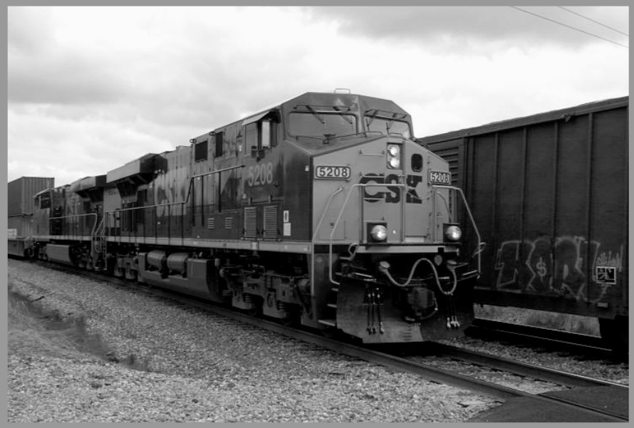
CSX intermodal, Q121, passes manifest Q556 at the south end of Latham siding. Power for the intermodal is a pair of new environmental friendly GE locomotives. ES44DC 5208 leads and 5240 trails. These are 6 axle, 4400 hp, DC drive locomotives. October 7, 2005 digital image by
