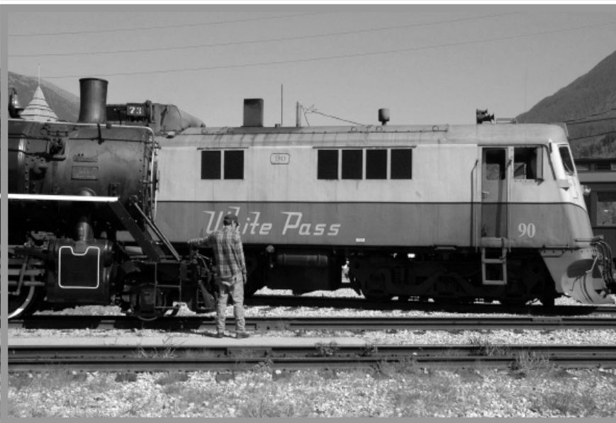
A Baldwin narrow gauge Mikado (2-8-2) was shuffling passenger cars in the Skagway yard of the WP&Y RR. Waiting it's turn for a run up the mountain to White Pass is a custom built GE locomotive with a unique shovel nose. These GEs with 950 hp prime movers are used in sets of 4 for the passenger trains running from Skagway to White Pass. digital image by Bob
