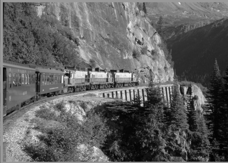
Three Alco (MLW) six axle, narrow gauge diesel locomotives pull an excursion train over roadbed hacked out of the mountainside on the way from Skagway to White Pass. The railroad climbs some 3000 feet in about 20 miles and was built during the Alaska Gold Rush. digital image by Bob
